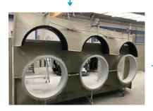
REMOVING FROM THE MOULD
